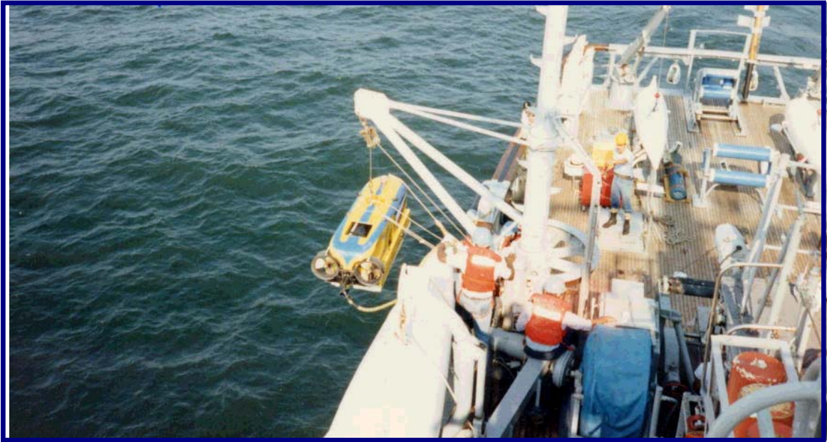
LAUNCH WITH THE STARBOARD QUARTER CRANE
